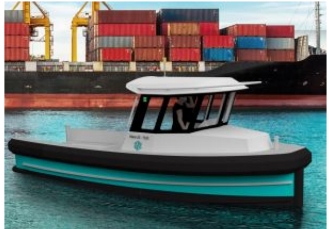
The NanoAir has a 6 mm thick aluminium hull with 40 mm thick rub-rails
